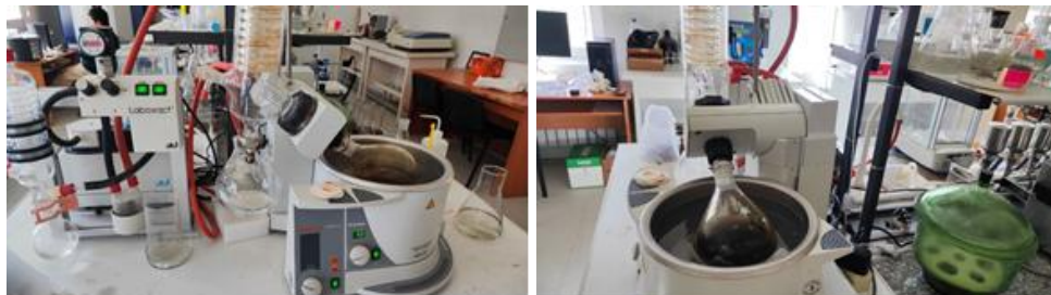
Figure 2. Separation of alcohol from the extract in a rotary evaporator.
